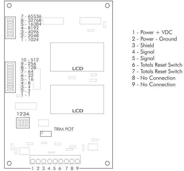
Connector Pin-out Diagram
