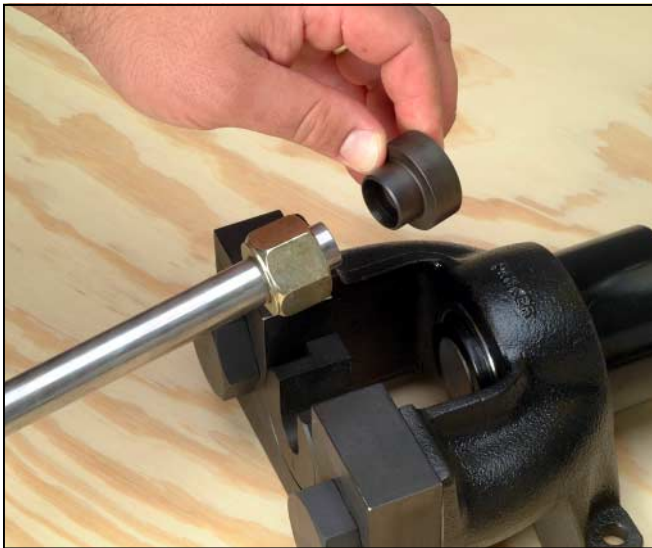
Step 9 Remove the Tube Lift out the tube with preset ferrule and inspect it according to the procedures shown to the right.
