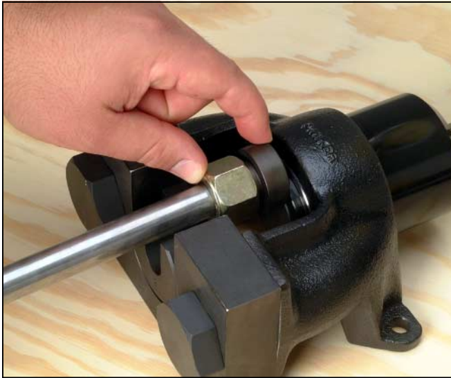
Step 7 Position the Assembly for Presetting Place the tube in the slot of the nut support.
