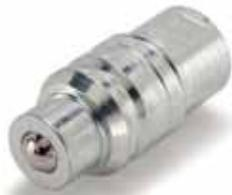
**5070-4, Male Tip.** Fits I-H 544788R1 and Pioneer 4057-4 female bodies. Ball style valving. Heat treated and zinc plated for resistance to wear and corrosion.
