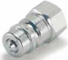
**SM-502-8FP, Male Tip - replaces 4610-4.** Connects with Allis-Chalmers 255018 and similar couplers. Has positive sealing poppet valve. Case hardened for wear resistance, zinc plated for corrosion protection.
