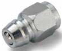
**\* 5060-4, Male Tip.** Fits John Deere AR47331 sleeve-type female bodies. Has durable chrome alloy precision ball valve. Induction hardened at the locking groove to minimize brinelling, and zinc plated for corrosion protection.
