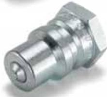
**5080-4, Male Tip.** Connects with J I Case A28542 and similar couplers. Has positive sealing poppet valve and shielded valve retainer to prevent flow checking. Case hardened and zinc plated for long service.
