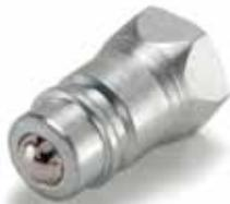
**8010 Series Universal Male Tip.** The standard male tip of the agricultural industry, Rugged, reliable ball valve and induction-hardened locking ball groove. Shielded valve plus valve stop eliminates flow checking when used with connect-under-pressure type couplers. Tapered hex design for easy identification.
