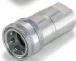
**4057-4, coupler.** Connects with I-H 544787R91 and Pioneer 5070-4 male tips. Interchange for I-H 544788R1. Has single-acting sleeve; trapped pressure must be released to make connection. Precision ball-check valving. Zinc plated.
